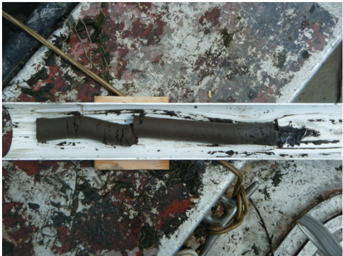
Photograph 10. Representative core sample (Sample 4A, shoreward of Lake Line). Top of core is at right.
