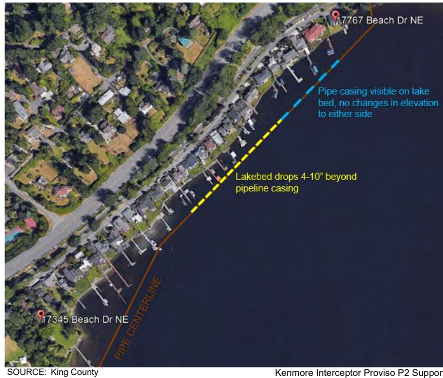
Figure 15 ROV Inspection Observations King County Environmental Lab – Oct. 2, 2019
